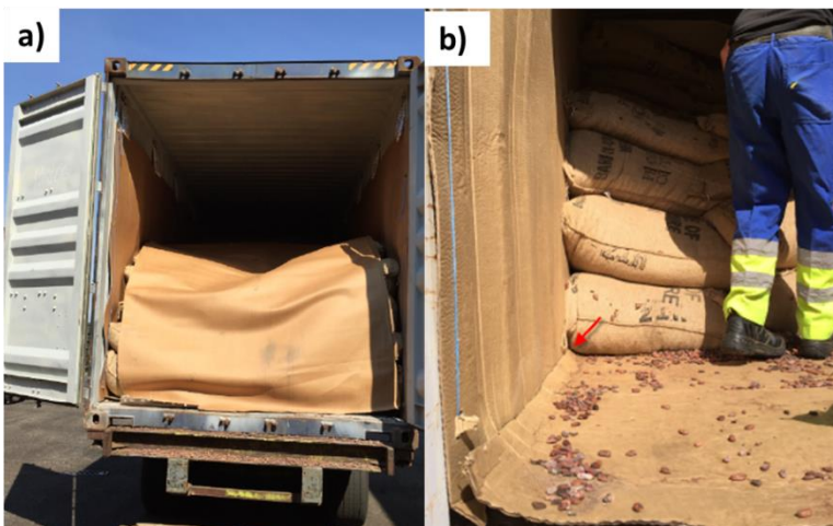
Figure 2. Photo of a) interior of the container; b) expansion of the contact between jute bags and cardboard on the bottom
